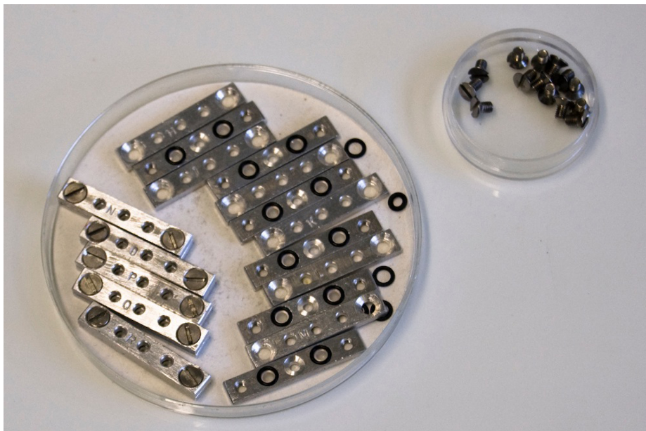
Figure 1. Custom-made 3-well chamber designed for freeze substitution. On the right are the bottom parts of the holders with 2 wells per holder fitted with an O-ring and on the left are the top parts to be screwed on after loading.
